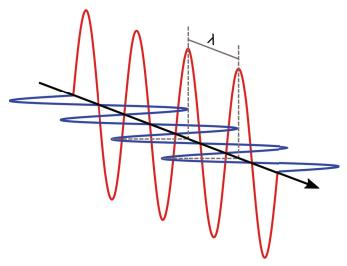
**Figure 1** Electromagnetic excitations are made up of a wave of electrical energy (red) together with wave of magnetic energy (blue). The two propagate in the same direction, but are perpendicular to each other. The wavelength, usually represented by the symbol  $\lambda$ , is the distance between adjacent peaks of the two constituent waves and is inversely proportional to the frequency; that is, the number of undulations (or oscillations) up and down per second.
